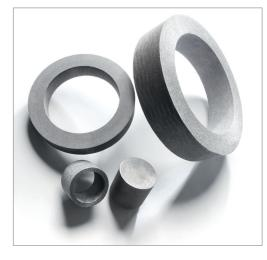
To meet any shape or process performance Bekaert sintered fiber regenerator is available in a wide variation of fiber diameters and alloys. The regenerator can also be swaged into assembly to ensure a tight fit or be sintered on your displacer cylinder or other engine part.
